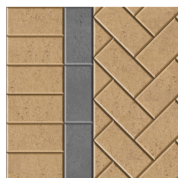
45° Herringbone with contrasting stretcher inlay and header
