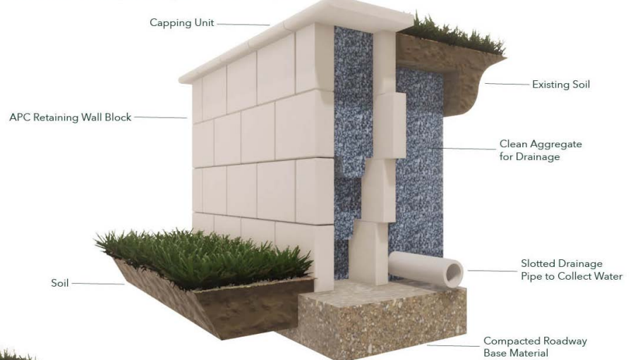
Vertical Retaining Wall up to .800mm High
