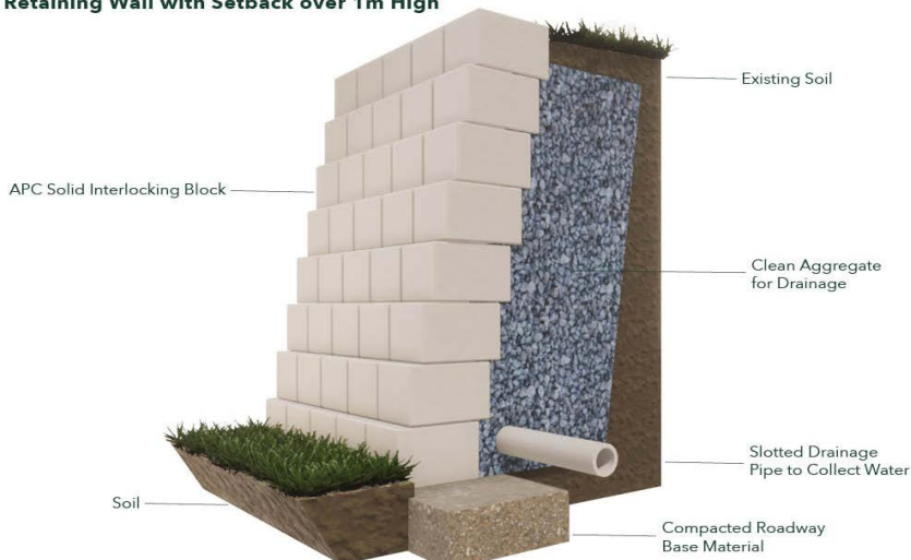
Retaining Wall with Setback over 1m High
